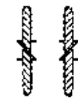
Yarns are spun and plied in either an 'S' or a 'Z' direction
